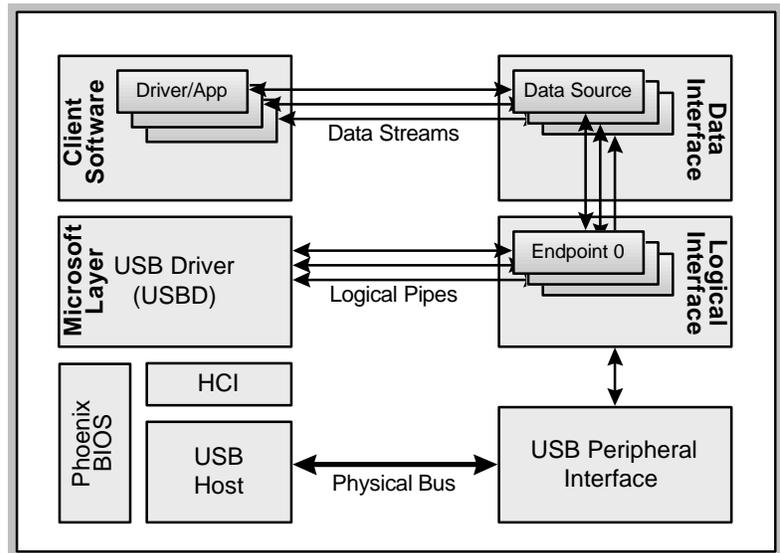
Figure 3 — USB Data Flow Architecture
