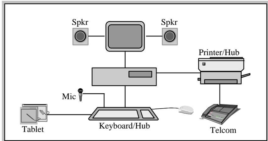
Figure 1 — Sample USB Device Configuration
